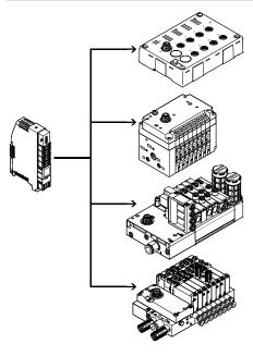
The IO-Link master module provides 4 external IO-Link interfaces. As well as transmitting the communication data, the IO-Link interfaces also transmit the power supply to the connected sensors and the load supply to the valves (or outputs). Both circuits are supplied separately with 24 V, using a separate reference potential. The load voltage supply is fed
