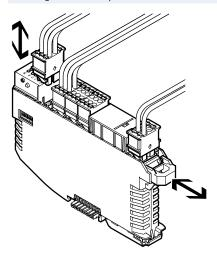
The terminal strips mounted on a module are held in position by central locking.
