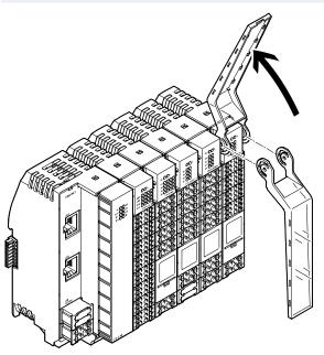
A hinged inscription label holder is available for the input and output modules and IO-Link master module. A matching label strip is inserted into the inscription label holder for labelling.
