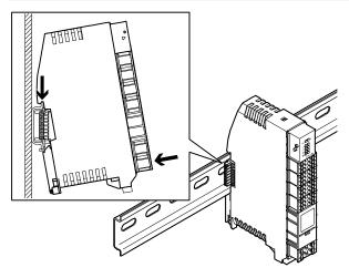
The module is attached to the H-rail or the electrical interlinking module and latched in place.
