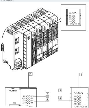
Each module has a row of LEDs for indicating the operating status of the module and of the connected sensors or actuators.
