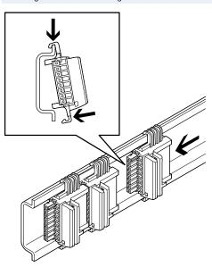
The electrical interlinking modules are clipped into the H-rail. They can be moved along the H-rail.
