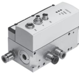
The 5/3-way proportional directional control valve for applications with Soft Stop and pneumatic positioning. Fully digitalised – with integrated pressure sensors, with new diagnostic functions. In sizes 4, 6, 8 and 10. Flow rates of 350, 700, 1400 and 2000 l/min.
