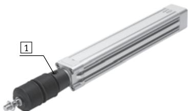
The protective bellows kit is a leak-free system. To prevent unwanted media from being drawn in, the supply and exhaust air must be ducted via a pressure compensation hole in the connection part [1].
