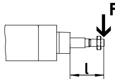
Maximum permissible lateral forces  $F_{y\max}$  and  $F_{z\max}$  on the piston rod as a function of stroke length l
