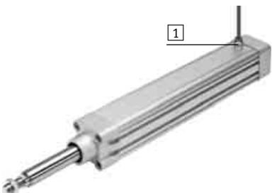
The electric cylinder to IP65 fulfils the specifications to IEC 60 529. Air is exchanged between the interior of the cylinder and the environment via a pressure compensation hole [1] in the cylinder barrel. This prevents negative pressure or excess pressure in the interior of the cylinder.
