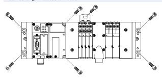
The MPA-F valve terminal is screwed onto the mounting surface using six M6 screws. The mounting holes are on the left-hand end plate (CPX) and on the right-hand end plate (MPA-F).
