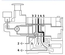
The reversible A regulator splits the working air in duct 1 and supplies the pressure upstream of the valve into duct 5 (the unregulated pressure from duct 1 is in duct 3). The regulated air is then supplied to duct 4. The valve is thus operated in reversible mode.
