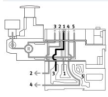
The reversible B regulator splits the supply air in duct 1 and regulates the pressure upstream of the valve in duct 3 (the unregulated pressure from duct 1 is in duct 5). The regulated air is then supplied to duct 2. The valve is thus operated in reversible mode.
