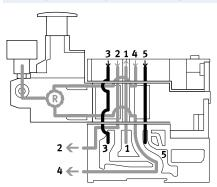
This pressure regulator regulates the pressure in duct 4 after the pressure medium flows through the valve. During venting, the exhaust flow in the valve is from duct 4 to duct 5 via the pressure regulator.
