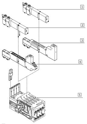
Vertical stacking components, MPA2
