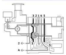
This pressure regulator regulates the pressure upstream of the valve in duct 1. Ducts 2 and 4 thus have the same regulated pressure.
