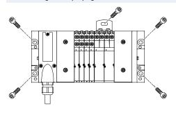
The MPA-F valve terminal is screwed onto the mounting surface using four M6 screws. The mounting holes are on the pneumatic interface and on the right-hand end plate.
