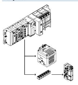
The optional string extension enables additional valve terminals and I/O modules to be connected to the fieldbus node of the CPX terminal. Different input and output modules as well as valve terminals can be connected.
