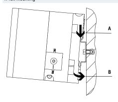
The MPA-F valve terminal is attached to the H-rail (see arrow A).
