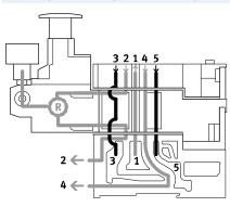
This pressure regulator regulates the pressure in duct 2 after the pressure medium flows through the valve. During venting, the exhaust flow in the valve is from duct 2 to duct 3 via the pressure regulator.
