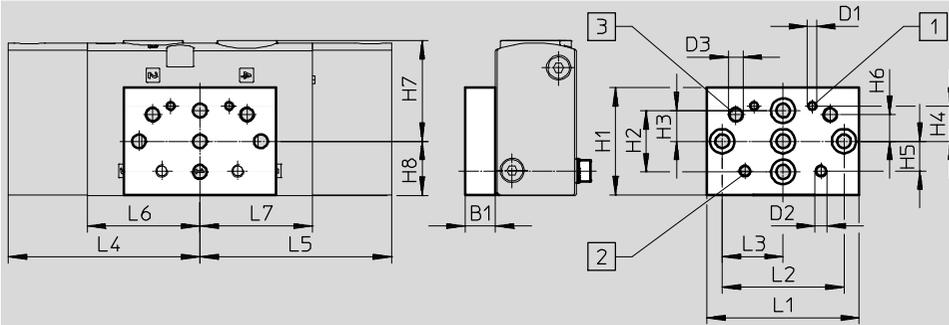
1 Mounting hole for size 20      2 Mounting hole for size 25      3 Mounting hole for size 30
