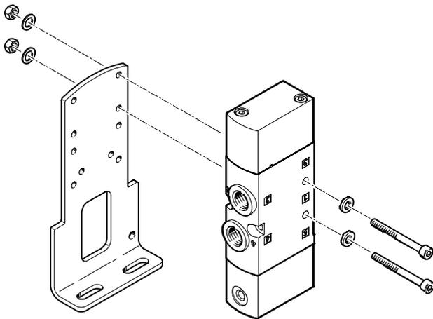
For mounting individual valves on a flat surface, e.g. aluminium profile systems. The pneumatic valves are provided with two through-holes for attaching to the foot mounting VAME-B10-...-A.
