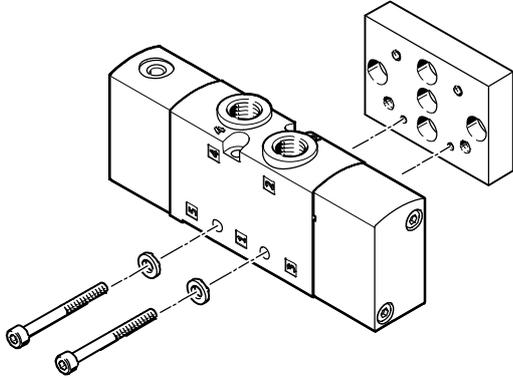
For mounting individual valves on a flat surface, e.g. aluminium profile systems. The pneumatic valves are provided with two through-holes for attaching to the wall mounting VAME-B10-20-W.
