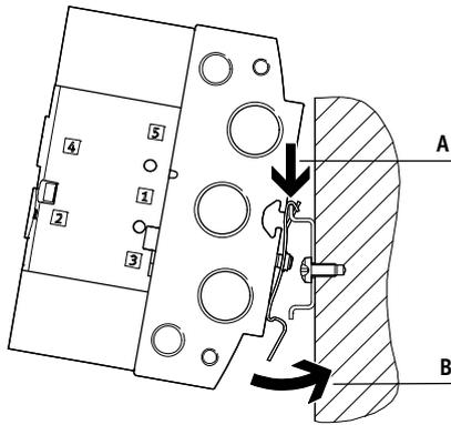
The H-rail mounting VAME-T-M... consists of two mounting clips. These are screwed to the manifold block on the left and right.
