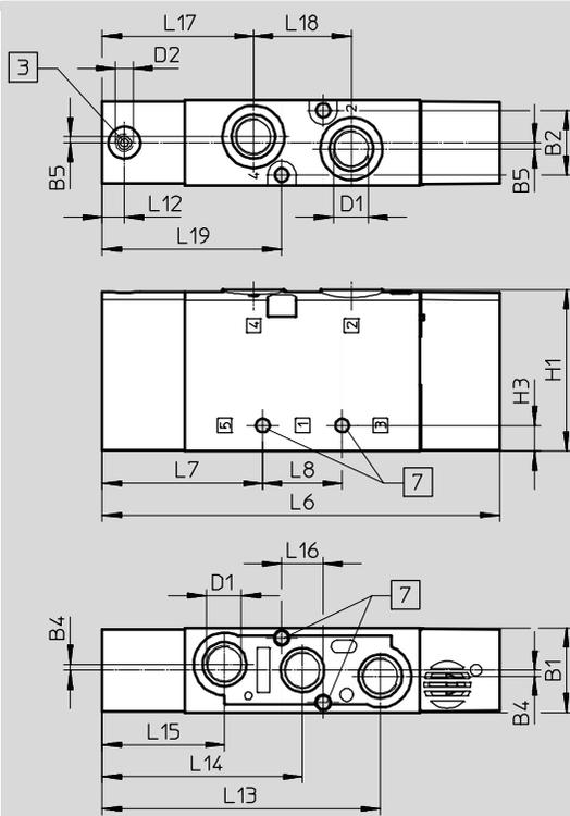
**3** Port 14: pilot air      **7** For mounting screw M4
